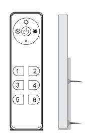
Place the remote control onto the magnet holder.
